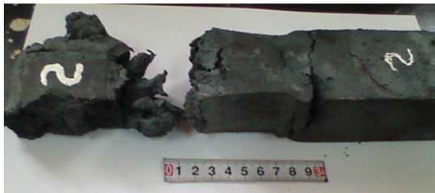
Figure 2: Alloy 0.02B Steel Couldn't Be Forged
